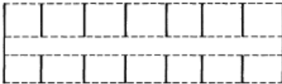
(a) Cross-walls without longitudinal walls: unstable
